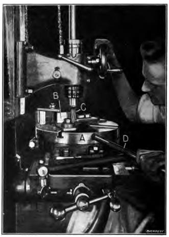
Fig. 14. Milling Segments for Pole-piece Punch
